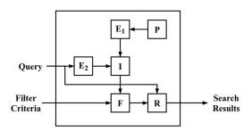
P: Patent Database, E<sub>1</sub>: Patent Encoder, E<sub>2</sub>: Query Encoder, I: Index (precomputed), F: Filter Sequence, R: Patent Ranker
